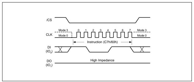
Figure 41. Chip Erase Instruction Sequence Diagram
