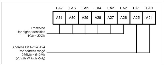
Figure 4e. Extended Address Register
