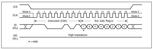
Figure 11. Write Extended Address Register Instruction
