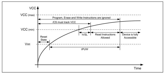
Figure 65a. Power-up Timing and Voltage Levels
