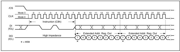
Figure 10a. Read Extended Address Register Instruction
