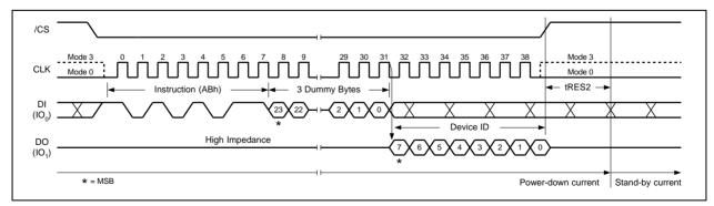
Figure 45b. Release Power-down / Device ID Instruction
