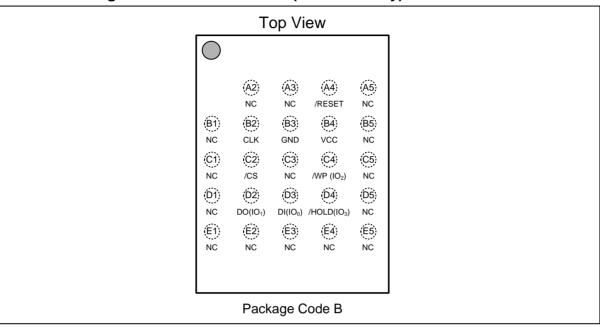
Figure 1c. W25Q512JV Ball Assignments, 24-ball TFBGA 8x6-mm (Package Code B)
