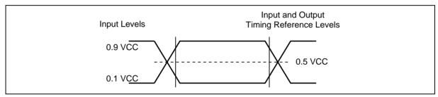
Figure 66. AC Measurement I/O Waveform
