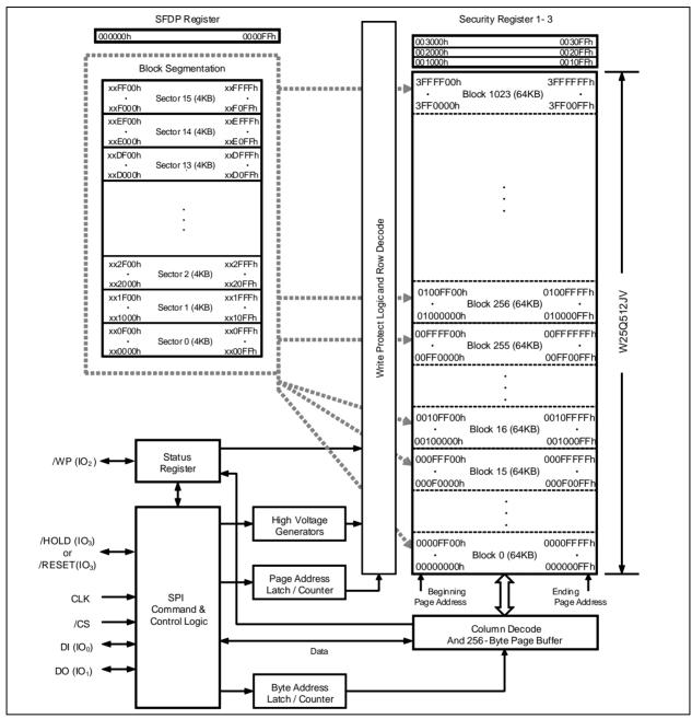
Figure 2. W25Q512JV Serial Flash Memory Block Diagram
