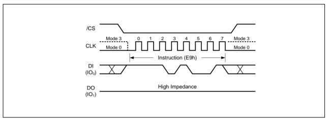
Figure 13. Exit 4-Byte Address Mode instruction
