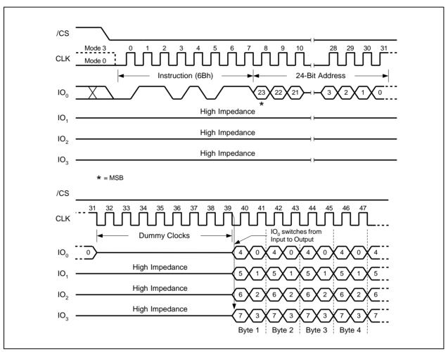
Figure 21. Fast Read Quad Output Instruction
