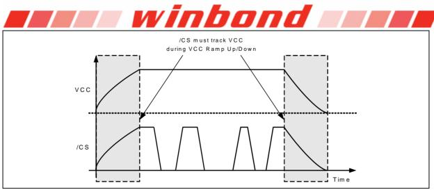
Figure 65b. Power-up, Power-Down Requirement
