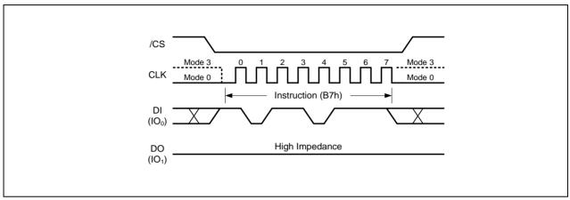
Figure 12. Enter 4-Byte Address Mode instruction
