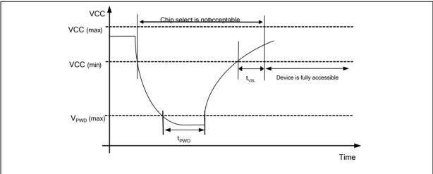
Figure 65c. Power Cycle Requirement
